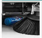
The 'flap-raising' device is activated directly from the driver's seat. It allows the central brush to pick up even the bulkiest and most obtrusive waste.
