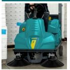
The car-like steering, the great visibility offered and the turning radius of only 1,050 mm make the RIder Lift an extremely agile and versatile machine.
